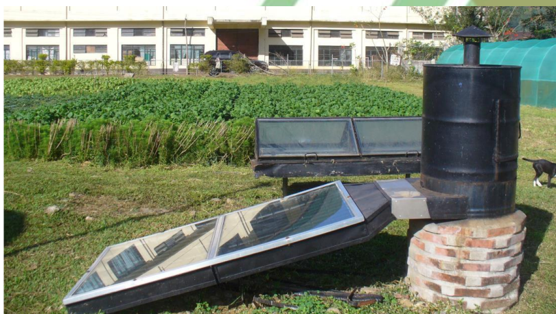
Figure 5. Fabricated solar dryer
