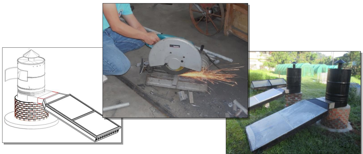
Figure 3. Flow of fabrication
